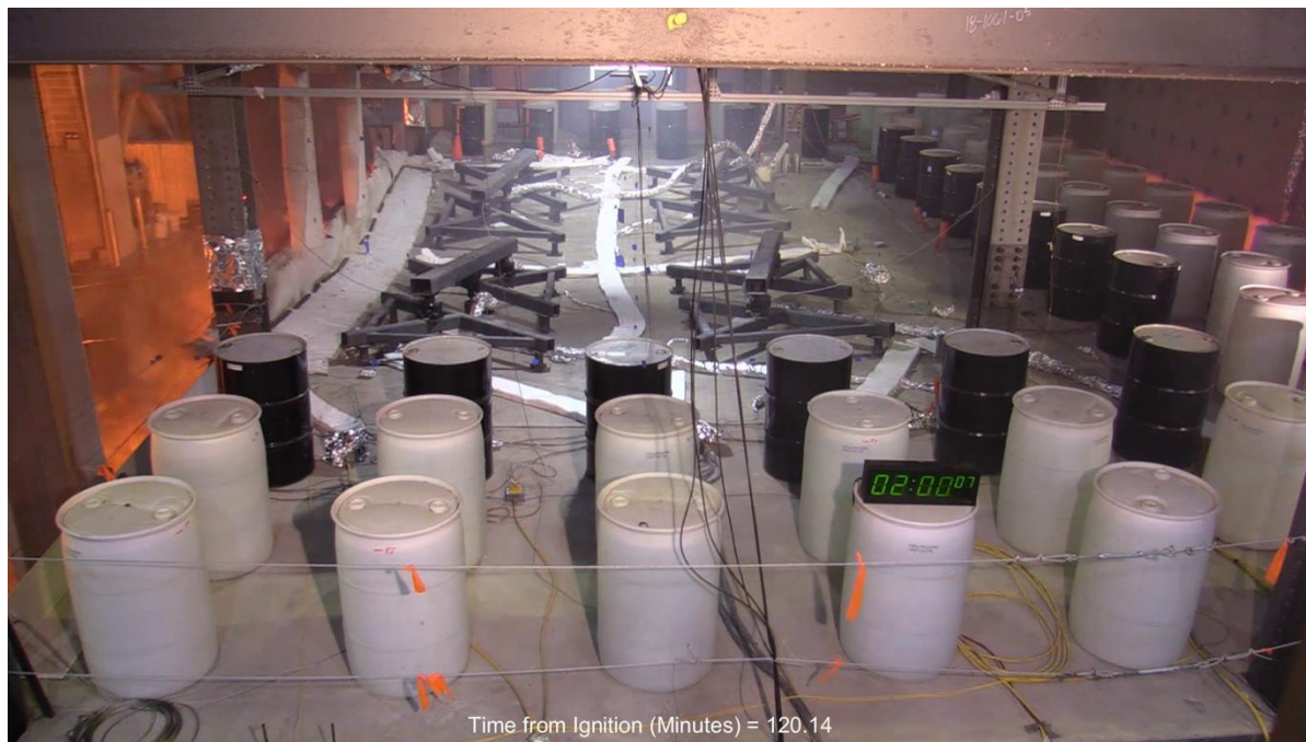
Fig. 63. Video snapshots showing the test floor at 15 min and 120 min after fire ignition.
