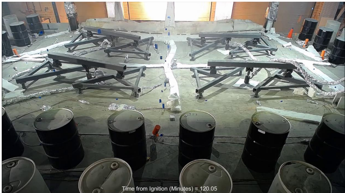
Fig. 29. Video image showing top of the test floor at 120 min after fire ignition.
